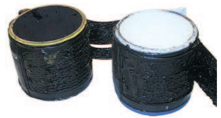
Fig. 4: DN 100 test body following peeling test
